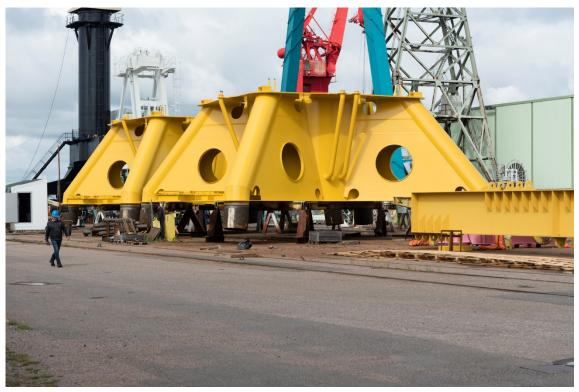
The last batch of the 30 heavy transition pieces for the offshore windmill foundations of the Beatrice wind farm in Scotland await shipping at Levator's pier. The large 150-ton objects connect the supporting tubes projecting into the seabed to the actual wind turbine tower and must endure the extreme weather conditions of the North Sea. During the torture test, Levator was able to produce one transition piece every five working days.
